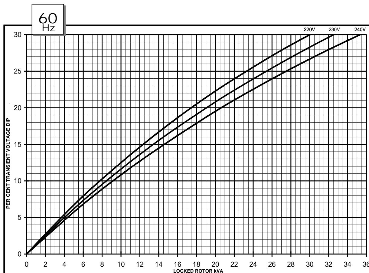
**Winding 311 Single Phase****WITH EBS FITTED**
