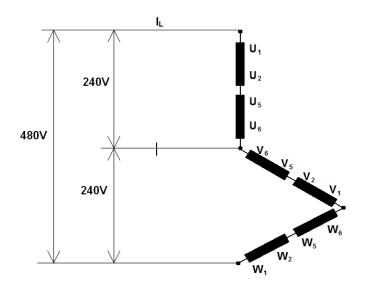
The maximum rating available from Winding 311 in this series zig-zag connection is limited to the following.
