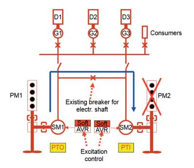
With two identical shaft generators, it is possible to swap over the PTO and PTI/PTH modes of operation from one side to the other.
