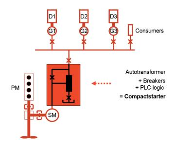
The shaft generator is started as an asynchronous motor with this method and therefore, requires some modifications to the excitation system of the machine. These modifications are explained later on in this AGN.
