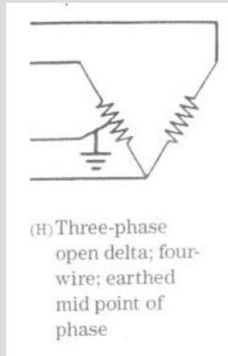
Note: the Code H configuration shows an open-delta, however; an AvK or STAMFORD alternator would always be connected in a full delta configuration.
