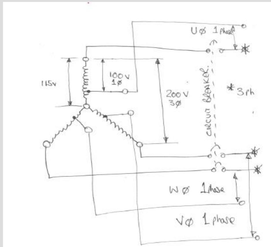
With the upgrade of alternators in the STAMFORD range, it has been decided to obsolete Winding 77. The outputs required for the Japanese national electrical distribution system, can now be supplied from STAMFORD alternators with the standard Winding 311, with a Parallel Star configuration.
