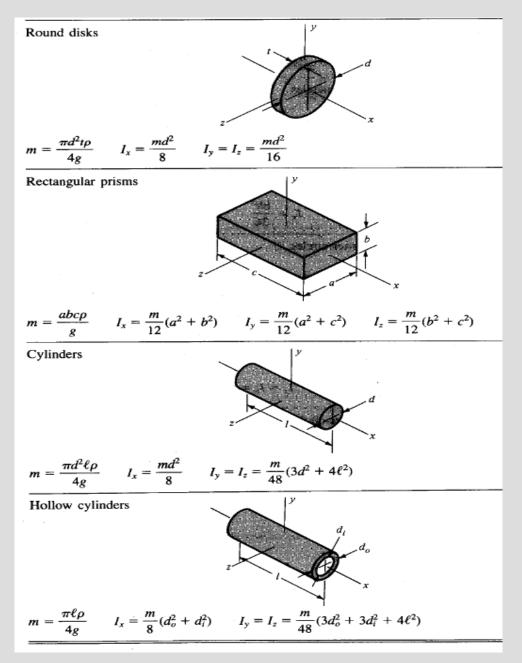
These inertias are then corrected due to their positions relative to the main rotor centreline. This is done using the parallel axis theorem.
