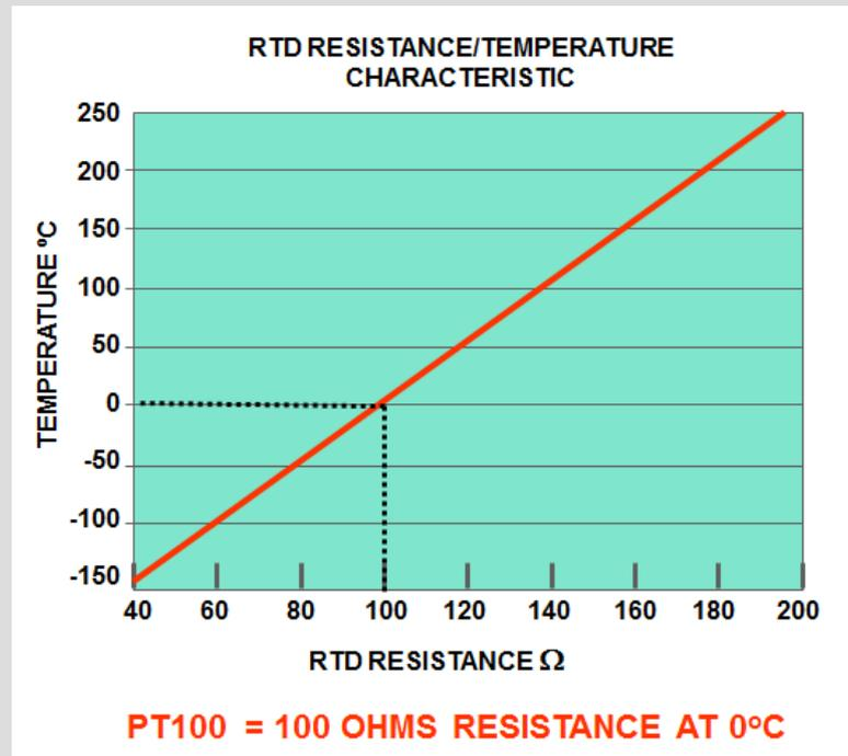
RTDs may be used for detecting temperatures in the stator winding, and they may also be used to detect temperatures in the alternator's bearings. Bearing RTDs are also type PT 100 devices, but of a different design to those used in stator windings.
