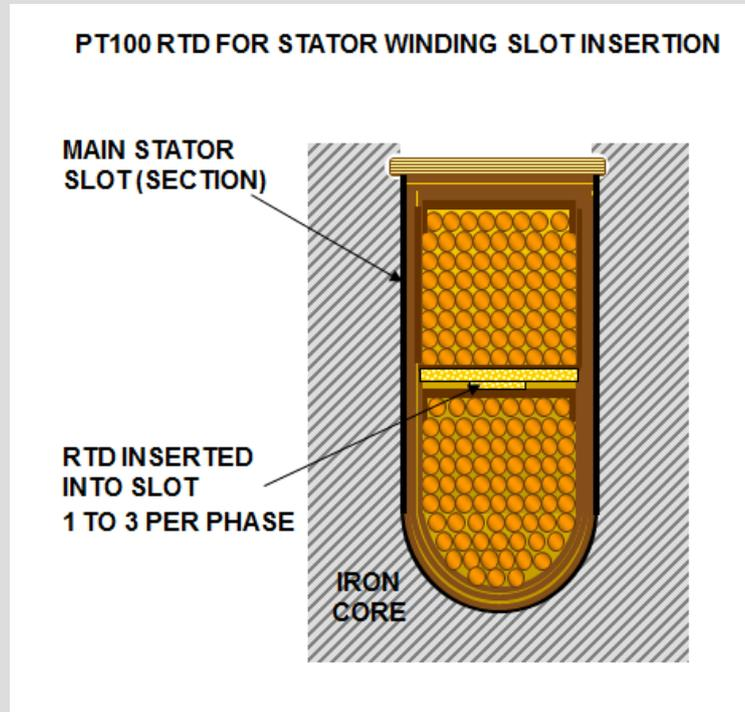
An alternators' winding temperature will be directly related to the kVA and power factor of the load, and so assuming an ambient of typically 30degC, an alternator will have 'roughly' the following component temperatures.
