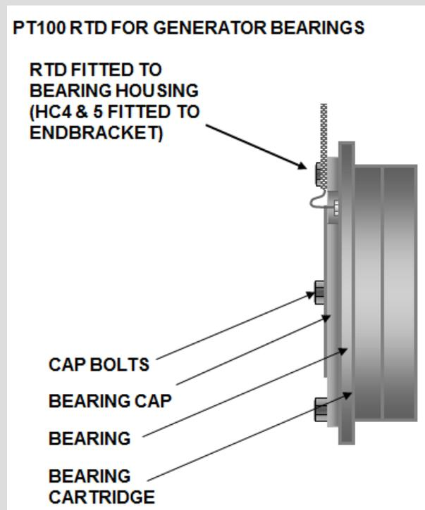
The temperature of a bearing is never a product of the bearing friction and generated heat, rather a temperature associated with the stator and rotor assemblies and the conducted heat from these two hot assemblies through the frame and end brackets into the bearing housing. In fact, a Drive End (DE) bearing's temperature is often governed by conducted heat from the engine components through the flywheel housing/alternator adaptor/ DE bracket assembly.
