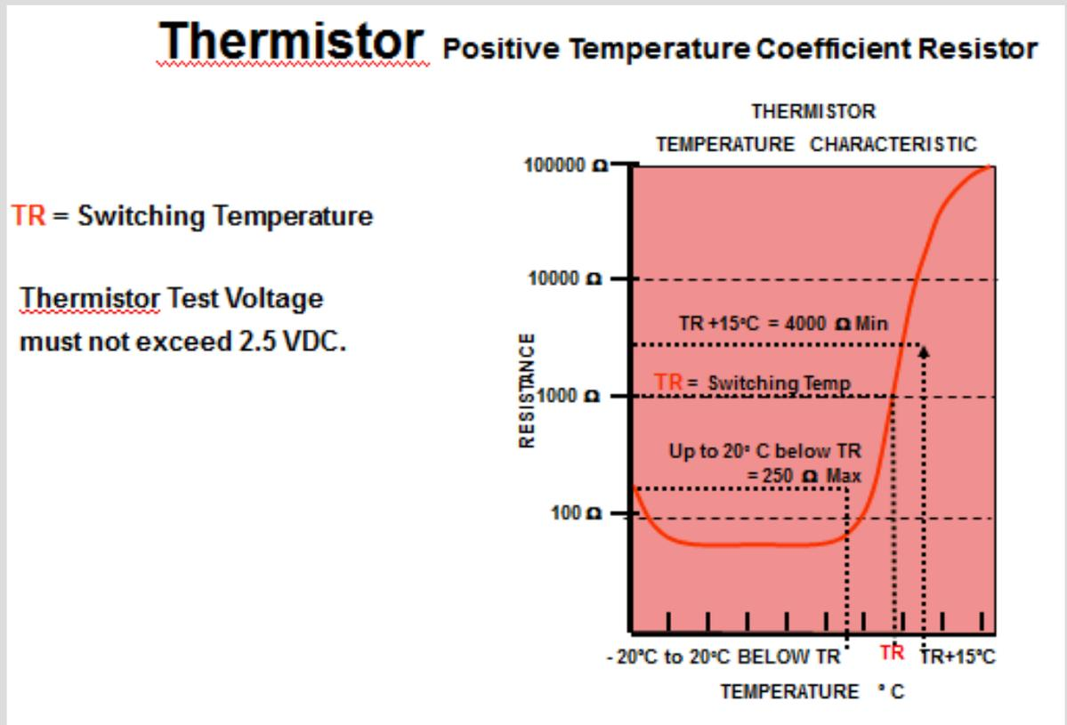
Typically, two of the above described thermistor schemes are incorporated, a system which operates at just above expected normal rated operating conditions and this scheme activates a control system function for triggering an ALARM.
