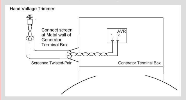
The suggested cable specification for this example is: 0.75mm2, 3A/500Vac minimum screened and jacketed twisted-pair.
