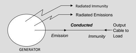
Conducted noise is at low frequency, typically 0.5 < 30 Meg Hz. Radiated noise is at higher frequency.
