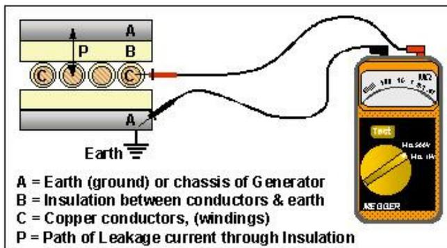
The high voltage causes a current to 'leak' through the insulation system. This current produces an output reading on the Insulation tester ('Megger'), which is measured in Megohms (resistance to earth or ground). A normal value for a low voltage Generator winding should be higher than 1 Megohm to earth.
