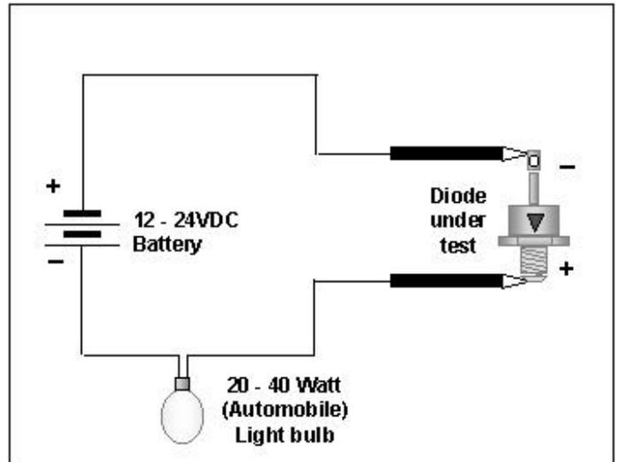
A good diode will light the bulb in only one direction. It should not light when test leads are reversed on the diode pin and base.
