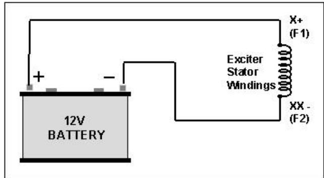
A variable source can be applied to the circuit, as shown: -
