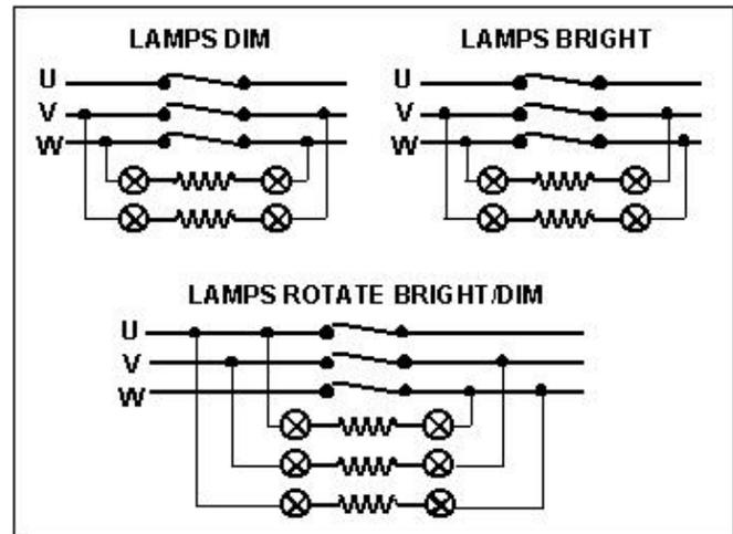
**NOTE:** If the neutral is solidly linked, then only one set of lamp/resistors is required, because the return path is through the neutral link. This, of course, only applies to the lamps dim or lamps bright connection, and not on the three lamp connection. Modern installations prefer to use semi, (check-sync.), or fully automatic synchronising equipment, which allows breaker closure only when conditions are correct.
