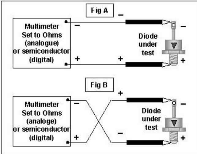
An electronic digital instrument will read true electron flow, hence the resistance polarity readings will be reverse to conventional current flow, i.e. forward and reverse readings will be reversed.
