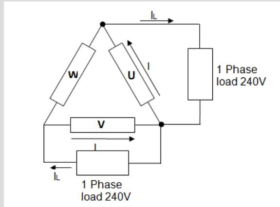
Each Single Phase load can be 240V X 100A = 24kVA
