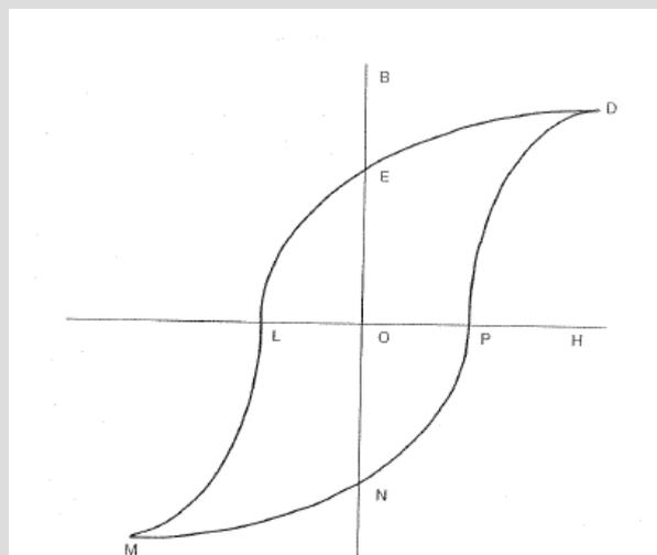
Note how once magnetised, the lamination steel retains a level of stored magnetic field strength (O to E) and is commonly referred to as the materials **remanence**.
