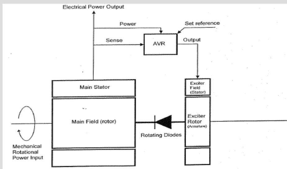
Then consider the normal mode of excitation control described below, which assumes the alternator is running at speed, the AVR is 'active' and therefore it can be said that the alternator is 'excited'.
