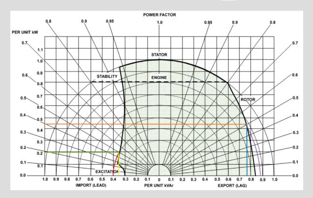
The above Op Chart is in fact based on a (half) circle diagram. The P vector is the central vertical radial line (12 o'clock), with the lagging Q out to the right (3 o'clock) and the leading Q out to left (9 o'clock). Around the clock face there are radial lines, against is assigned a power factor.
