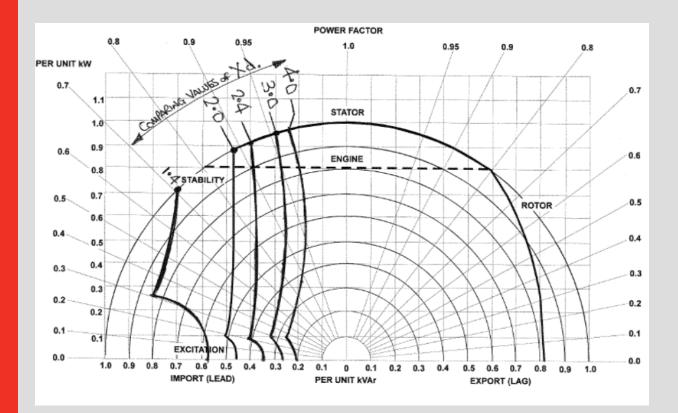
For example; the above Capability Diagram has been created for an alternator rated at 100kVA. From that alternator's technical data sheet, we can read the synchronous reactance (Xd) value is 2.0pu at 100kVA. The load to be considered has been identified as being 70kVA at 0.8 pf lead.
