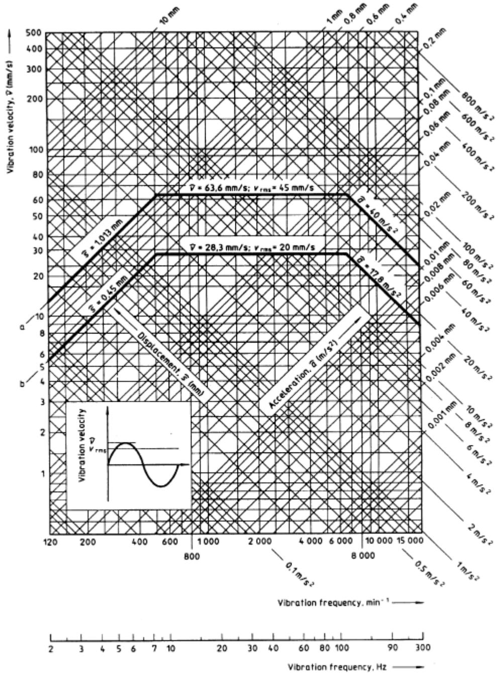
Examples for limiting curves for sinusoidal vibrations
