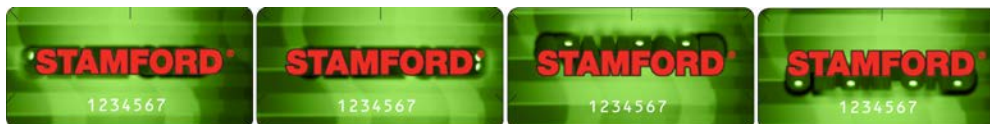
FIGURE 3. DOTS VISIBLE IN LEFT, RIGHT, UPPER AND LOWER VIEWS OF 3D HOLOGRAM
