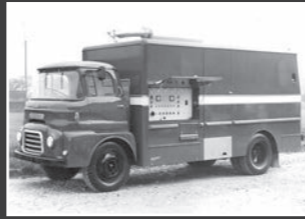
The 'L' range used in an Austin van, coupled to a Dale Electric set.
